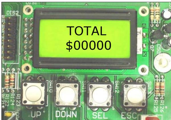
Navigation through the software's various menus is done using the LCD screen and the four pushbuttons located directly below it as an interface. Many things are accomplished within the software, including setting up the coin hopper and bill dispenser, setting the payouts, initiating the printing of an Audit Receipt (if a printer is installed), and accessing accounting and other diagnostic information.
